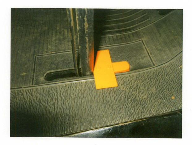
Once inserted it ensures that the car is in neutral and will stay there. Obviously while starting I pull back the emergency brake all the way but should the ratchet fail the worst that can happen is that the car which is in neutral creeps forward slowly as a result of drag between the high speed clutch plates which run in oil.
